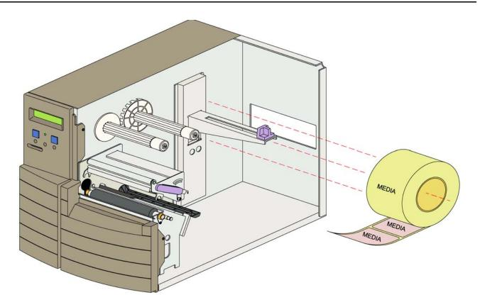
Figure 7-5a, Printer Loading Diagram
